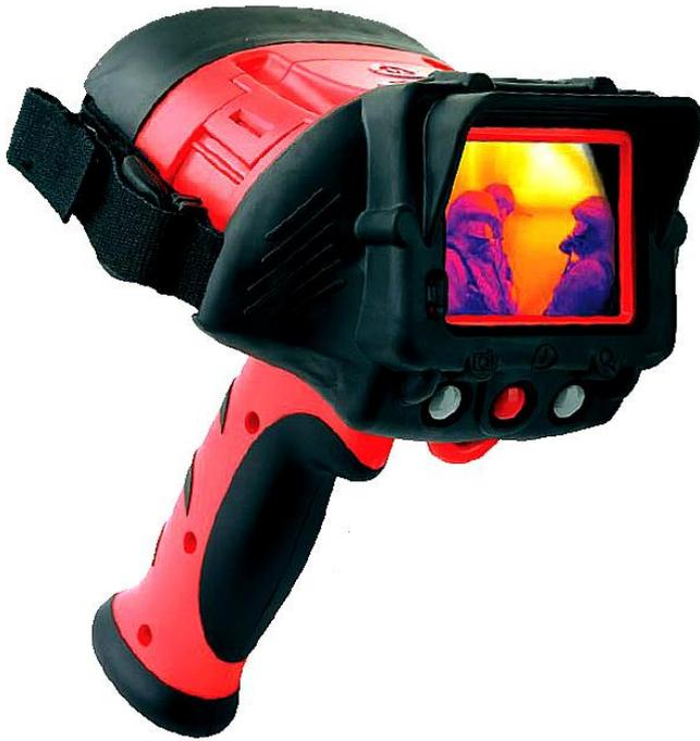
The Argus®4 series has been specifically designed to help fire fighters to see in conditions of zero visibility including complete darkness, and smoke. It allows them to identify and rescue casualties, locate hot spots and the seat or spread of the fire. They use an uncooled high-resolution 160 x 120 pixel, Amorphous Silicon (ASi) Microbolometer Detector.
